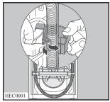
3. With a suitable spanner unscrew and remove the central rear bolt A. Slide out the relevant plastic spacer.
